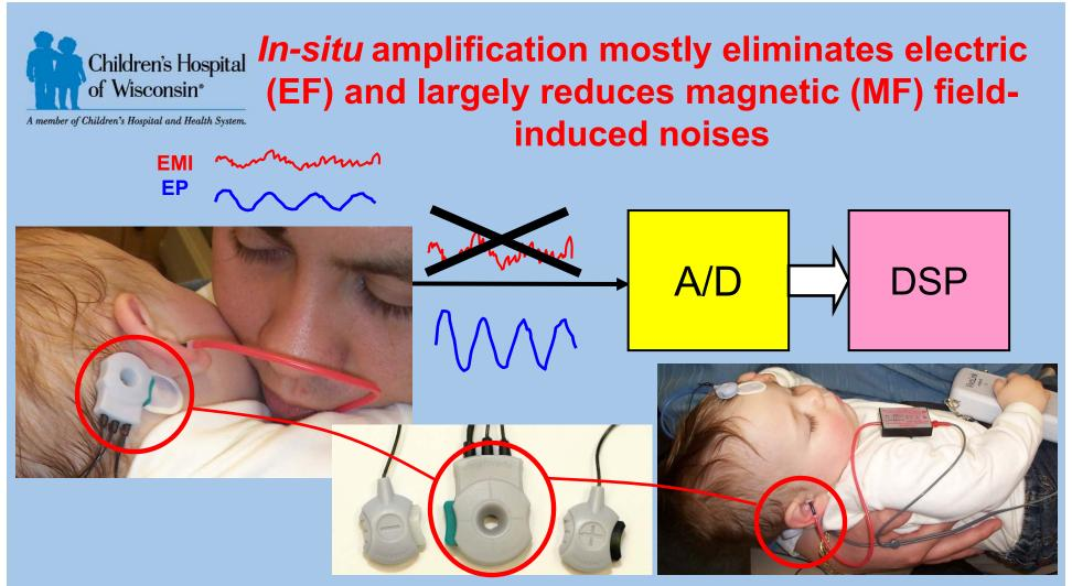
*In-situ, electrode-mounted* pre-amplifier, the Amplitrode<sup>™</sup>, eliminates the ground lead, with the other leads very short and shielded.
